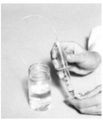
**5** Examine capillary tube to be sure there are no air bubbles.
